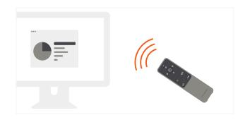
After ten minutes of inactivity, the remote will go into sleep mode. Press any button to wake.
