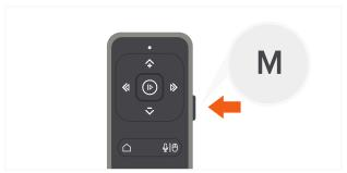
Enable the on-screen laser feature within PowerPoint or Keynote settings with the remote in Presentation mode (P).
