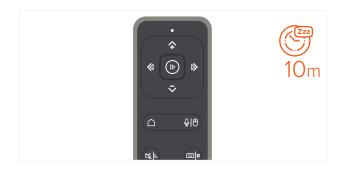
2 Enter pairing mode by press and holding the remote's Bluetooth button for ~3 seconds.
