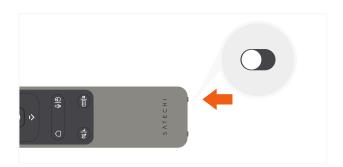
3 Select "R2 Remote" when it appears in your host device's Bluetooth settings to connect and finish the pairing process.
