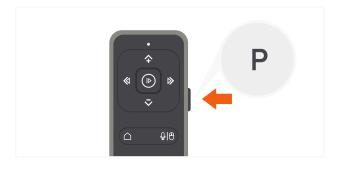
8 To recharge the remote, connect to a powered USB-C port using the included cable. Flashing red light indicates low battery. Red light will turn green when fully charged
